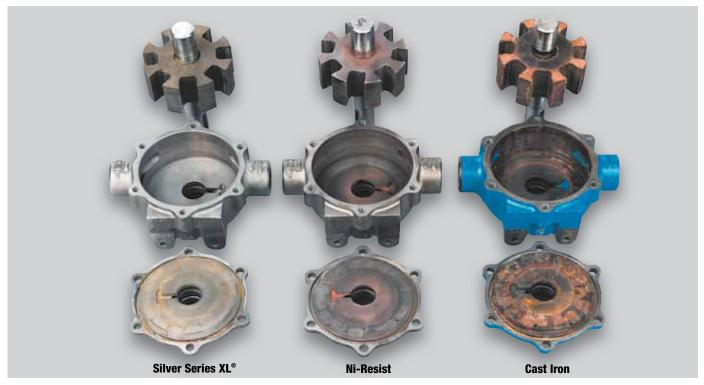
The three pumps shown above were photographed after being tested with a 30:1 mix of water and Roundup<sup>®</sup> herbicide. The Ni-Resist and Cast Iron indicate damage from pitting and corrosion, but the Silver Series XL<sup>®</sup> is in like-new condition after more than 1000 hours of use.
