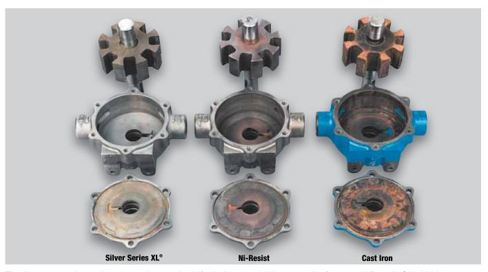
The three pumps shown above were photographed after being tested with a 30:1 mix of water and Roundup® herbicide. The Ni-Resist and Cast Iron indicate damage from pitting and corrosion, but the Silver Series XL® is in like-new condition after more than 1000 hours of use.
