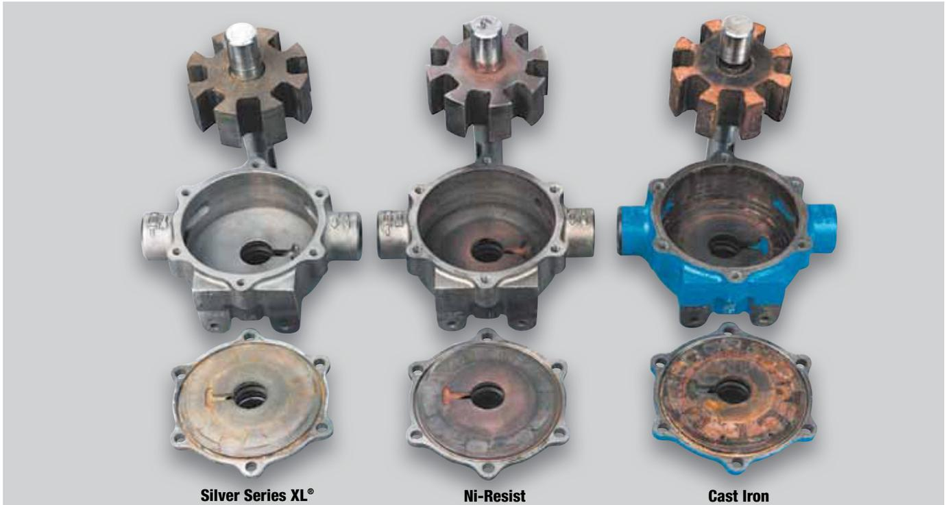
The three pumps shown above were photographed after being tested with a 30:1 mix of water and Roundup® herbicide. The Ni-Resist and Cast Iron indicate damage from pitting and corrosion, but the Silver Series XL® is in like-new condition after more than 1000 hours of use.
